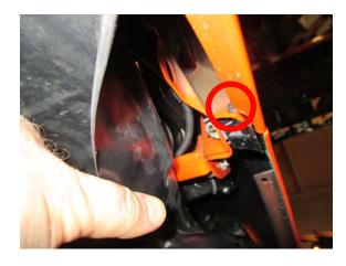
**Step 7:** With the splash shield removed, you can access the plugs for the turn signals and fog lights.
