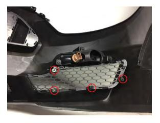
**Step 15:** Install the grille extensions from the front side of the bumper by clipping them to the grille.
