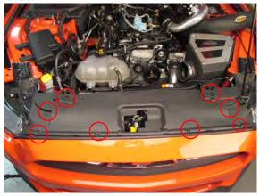
**Step 3:** Remove the 8 bolts securing the bumper cover to the rad support.
