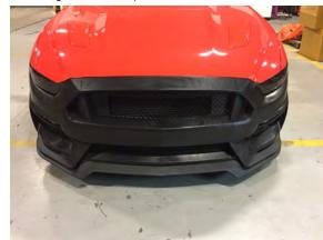
Step 20: It may be necessary to trim part of the chin spoiler in order to reuse the factory clip. Use wire cutters to cut away enough of the chin spoiler to slide on screw clips.
