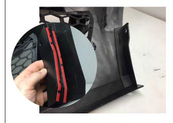
**Step 17:**Transfer the hood weather stripping from the factory bumper to the new bumper.
